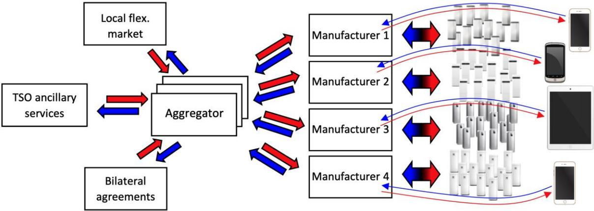
Figure 14: Overview of the communication flow from and to the heat pumps using the manufacturers cloud solution.
