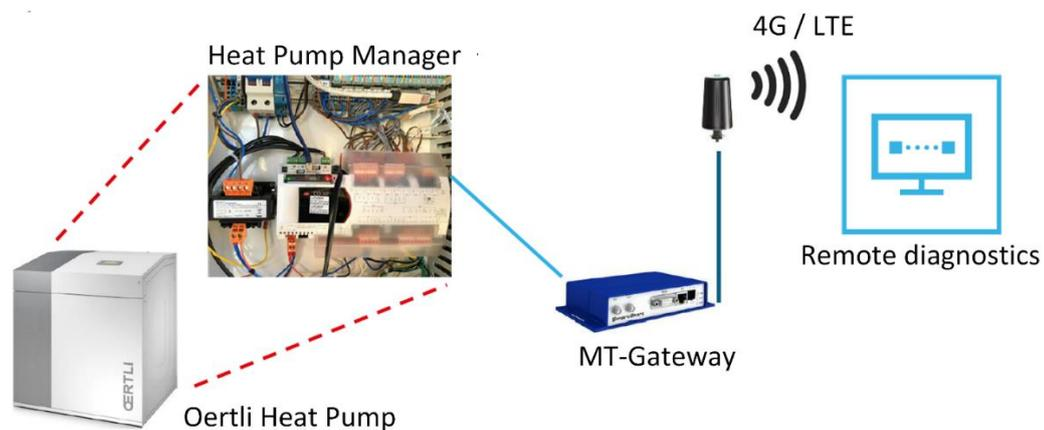
Figure 16: SmartGuard system setup (Di Cerbo, 2022)
