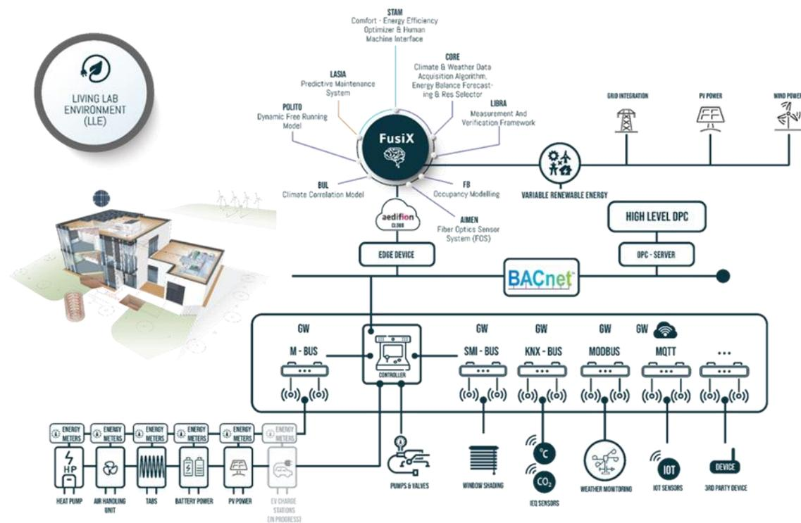
Figure 11: Data management architecture of the intelligent Energy Management System (cf. PRELUDE, Grant Agreement No. 958345)
