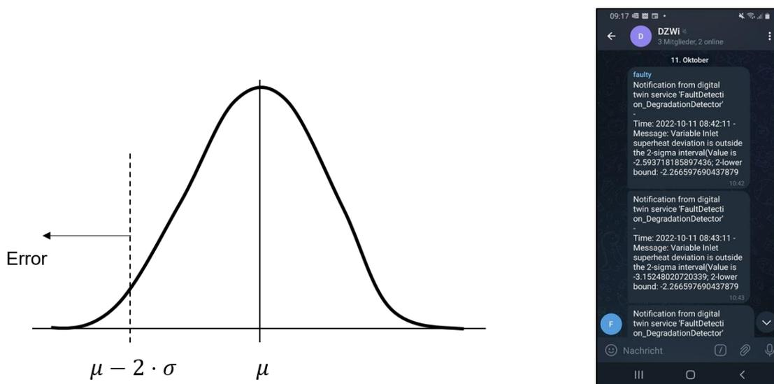
Figure 6: Left: Trained mean value and standard deviation of a certain system behavior. If (in this case) the value falls below the  $2\text{-}\sigma$  interval, an error is detected. Right: Output or notification when fault detection is triggered via the Telegram messaging service.
