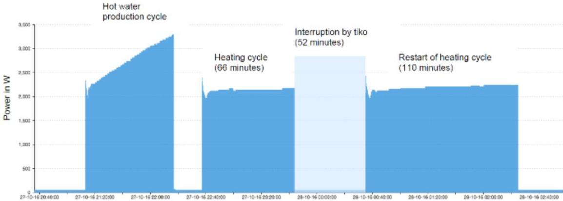
Figure 55: Heat pump cycle interrupted by tiko control
