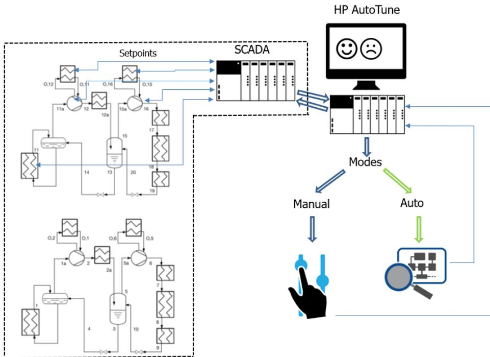
Figure 67: Diagram of the HP AutoTune concept.
