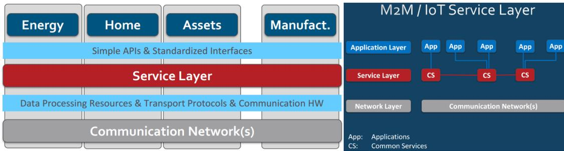
Figure 23: Functional architecture of oneM2M. Source: (Blanz, 2012).
