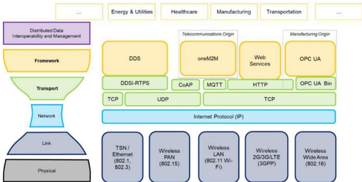
Figure 21: IIoT connectivity stack. Source: (IIC and I4.0, 2017)
