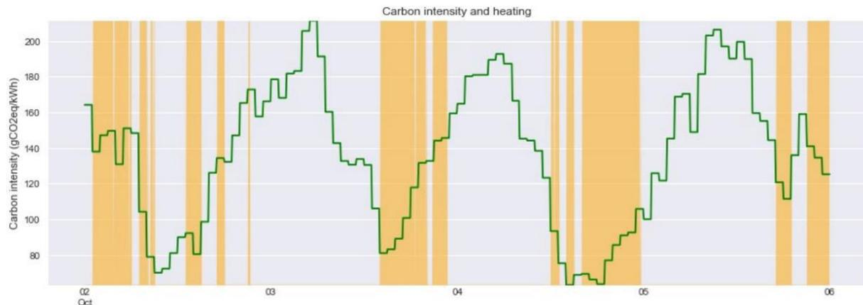
Figure 69: Predicted carbon intensity (green) and periods at which the heat pump is turned on (orange).
