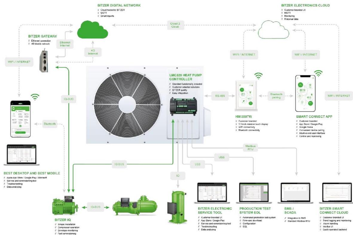
Figure 39: Overview of the Bitzer Heat Pump Ecosystem
