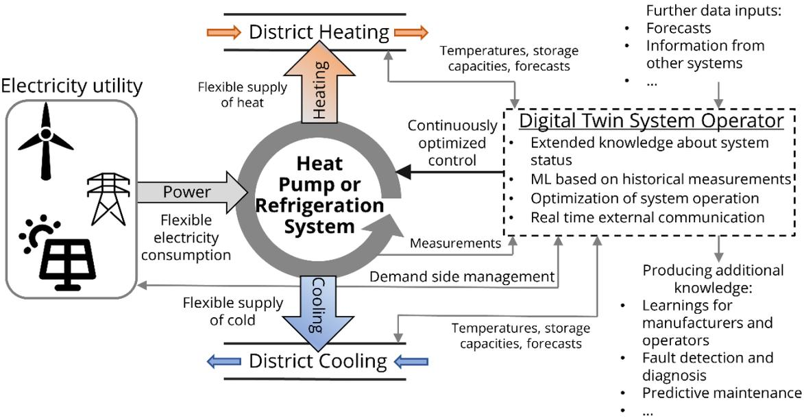
Figure 61: Diagram of the digital twin system operator.
