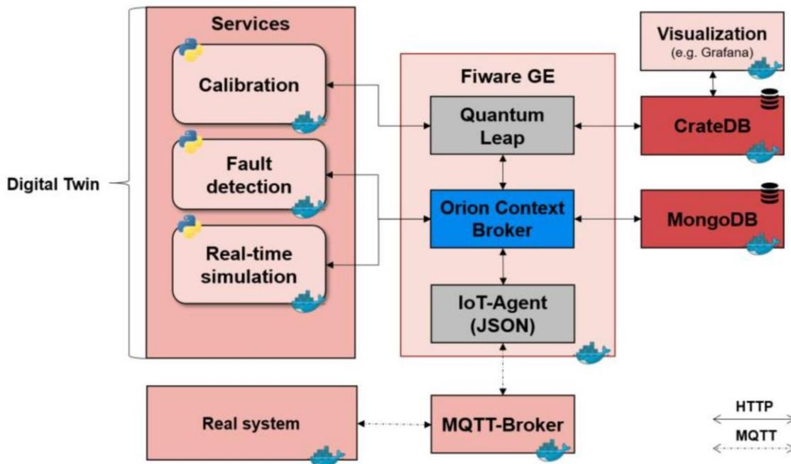
Figure 58: Fiware architecture for communication of virtual/real system and implemented services
