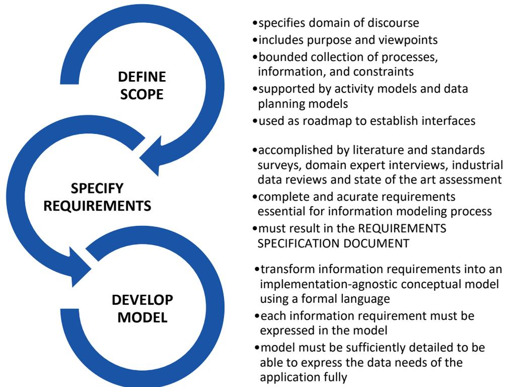
Figure 28: Information Model Development Process. Adapted from (Lee, 1999).
