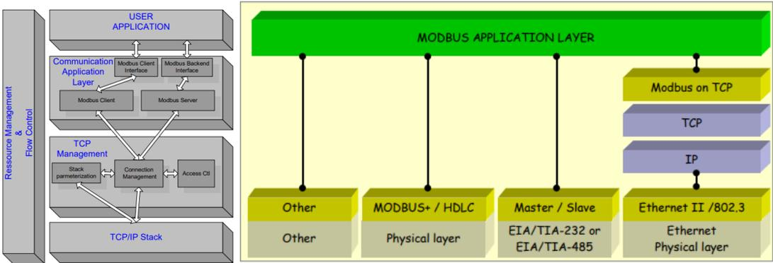
Figure 16: MODBUS Messaging Service Conceptual Architecture and communication stack. Source: (Bellardi & Neubert, 2015).
