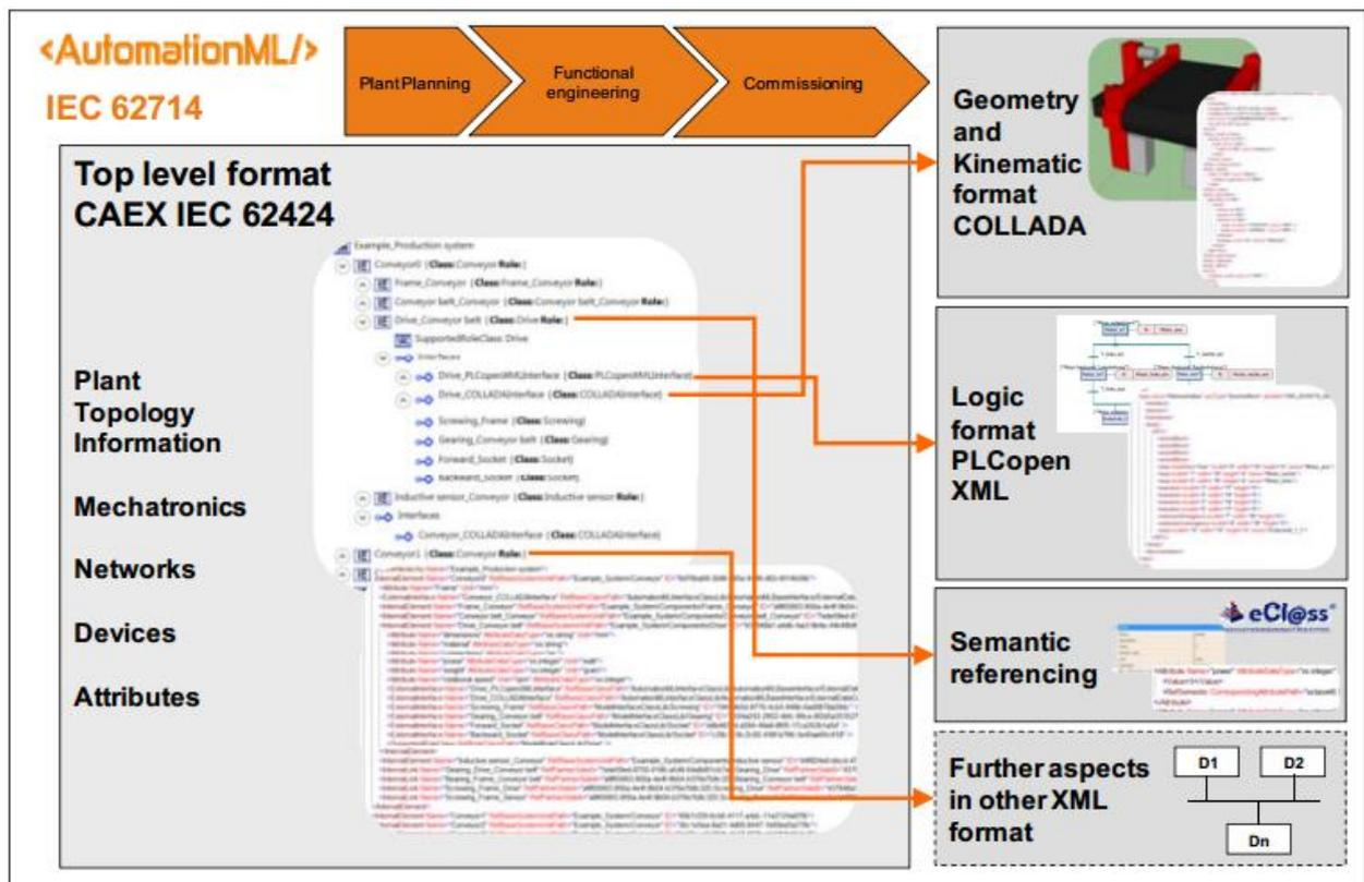
Figure 36: Structure of AutomationML Projects. Source: (Lüder, 2015).
