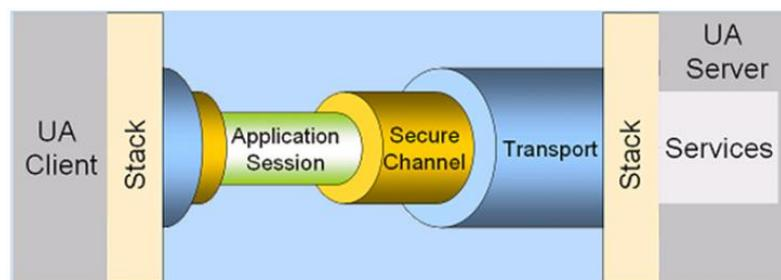
Figure 27: The client-server architecture of OPC UA. Source: OPC Foundation.
