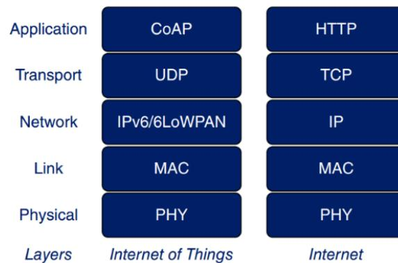
Figure 20: CoAP protocol stack vs. HTTP protocol stack.
