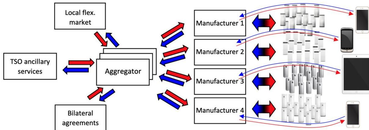
Figure 52: Overview of the communication flow for demand response from heat pumps using the manufacturers cloud solution
