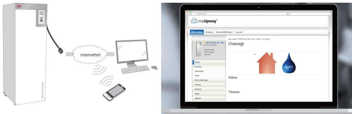
Figure 83: Representation of the interconnection between METRO THERM heat pumps and desktop through myUpwayTM (left) and homepage of the online service myUpwayTM (right).
