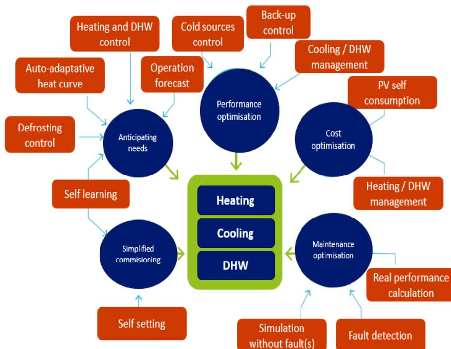
Figure 70: Use functions fulfilled by a smart heat pump
