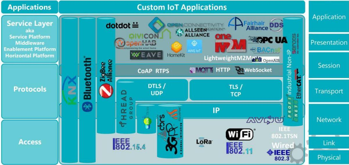
Figure 13: Technologies in IoT Stack. Source: (Blanz, 2012).
