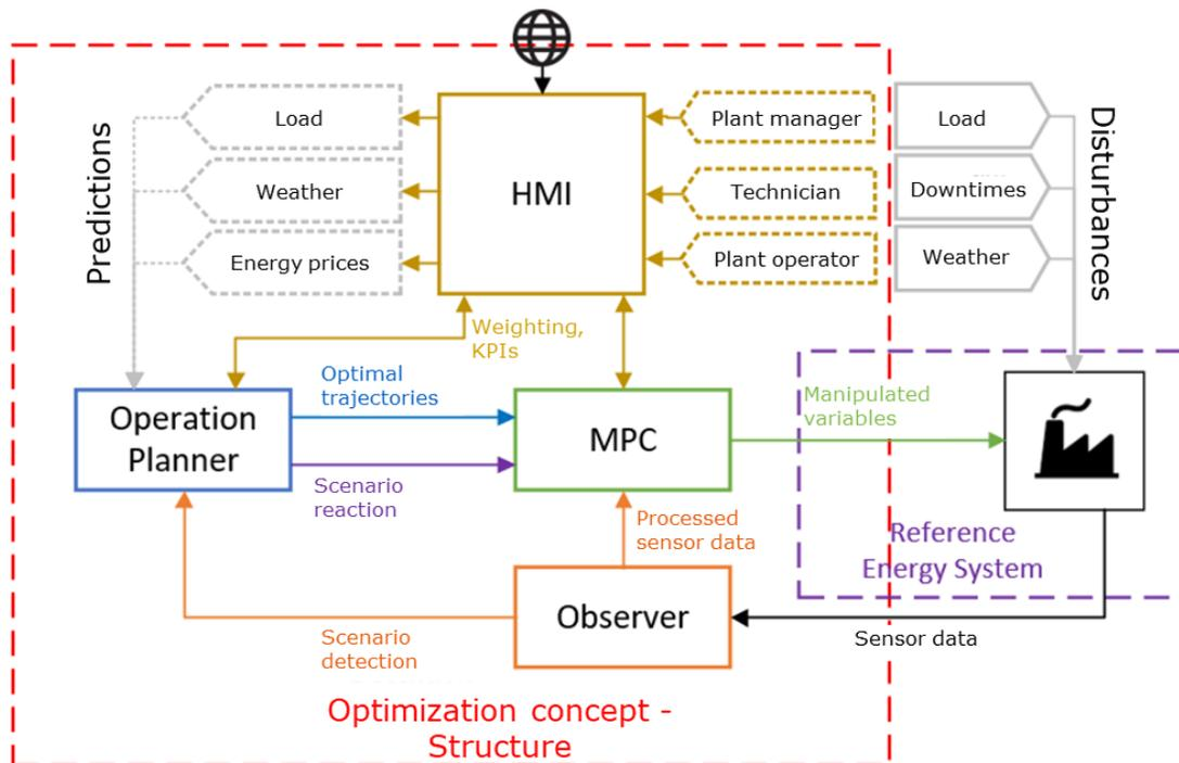
Figure 47: Visualization of the Energy Demand Control System EDCS
