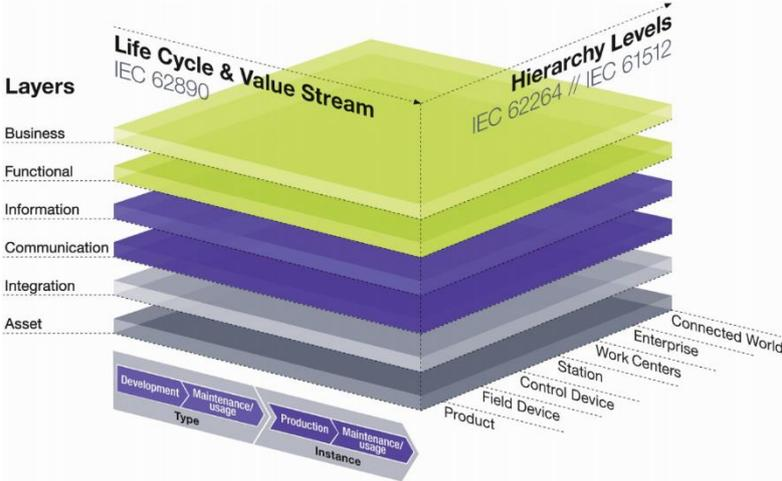
Figure 6: Reference architecture model Industry 4.0 (RAMI4.0).
