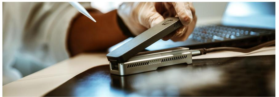
Figure 1: MinION device from Oxford Nanopore Technologies used for sequencing
