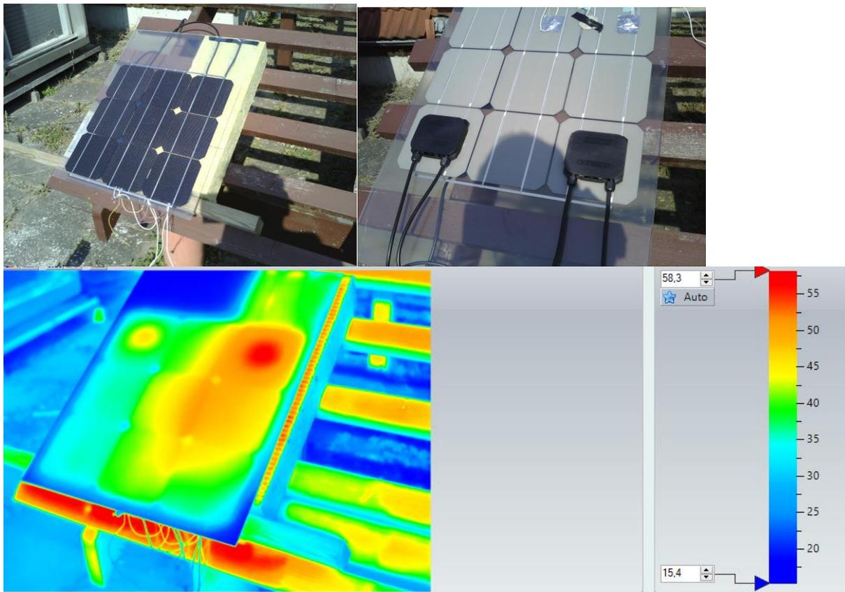
Figure 8 Thermal photo of the front glass (may not be exact but shows remarkable difference).
