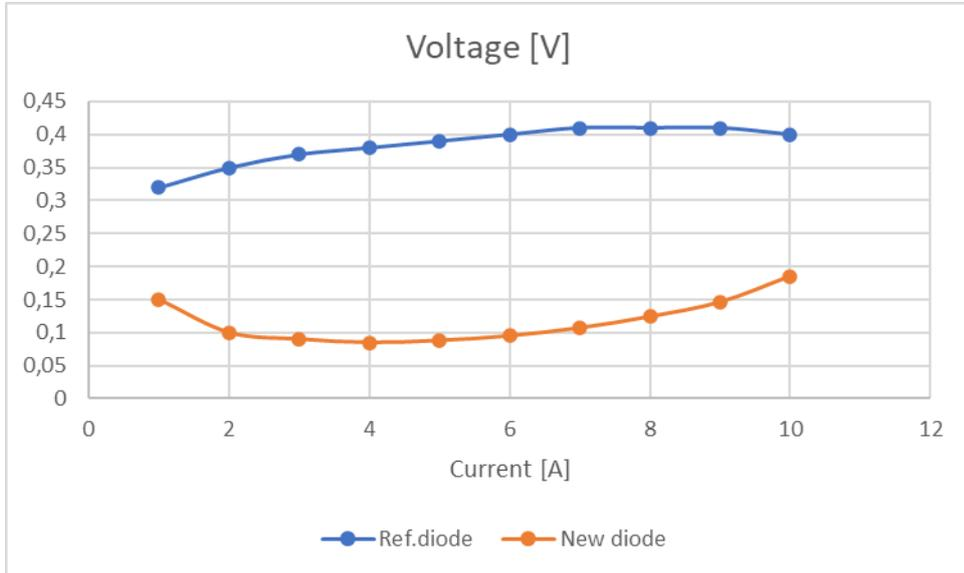
Figure 2 Comparison of voltage drop. The standard diode shows a fairly constant value of 0.35 - 0.4 V. The smart diode has its minimum voltage drop at medium load.
