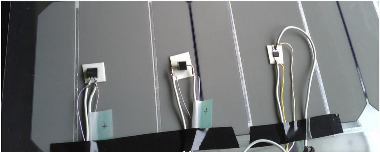
Figure 4 Mounting of three different diodes on a glass/Tedlar PV laminate. From left, it is active diode, standard diode, and flat diode (also Schottky). They are mounted on the module with double adhesive tape.
