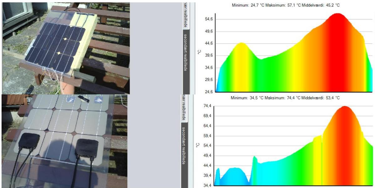
Figure 10 Temperature profile across the two junction boxes from front and rear.
