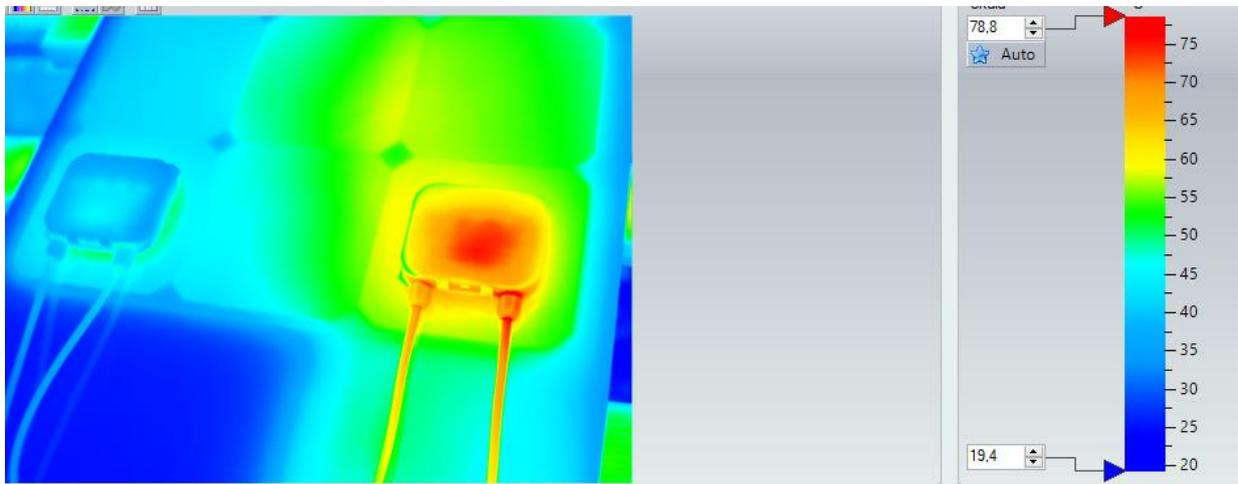
Figure 9 Temperature on the back immediately after removing insulation.
