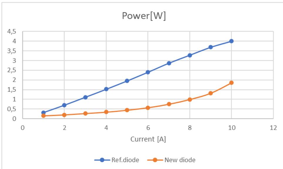
Figure 3 Comparison of power loss. The active diode has much lower loss, but it increases sharply at high current.
