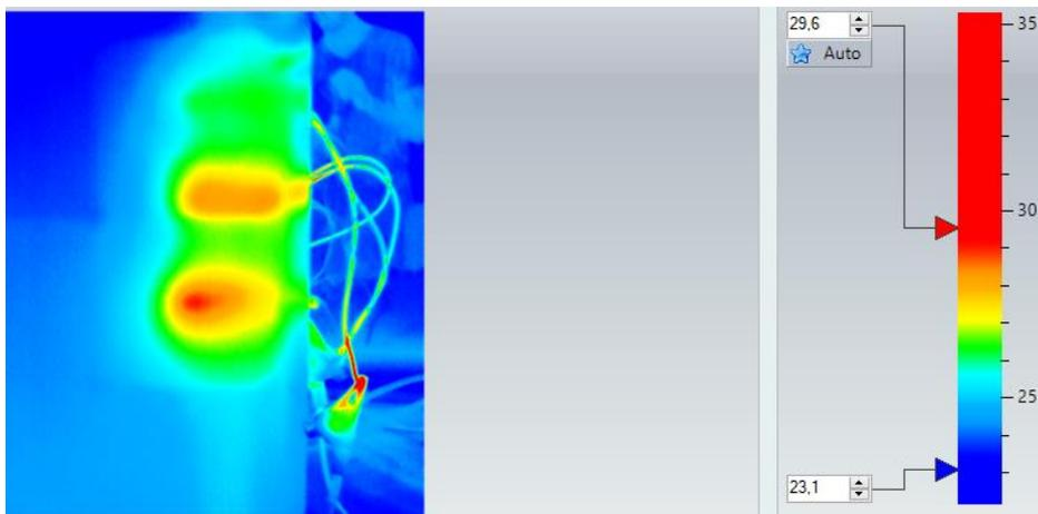
Figure 6 Thermal image seen from the front. The glass is warmest in front of the flat Schottky diode.
