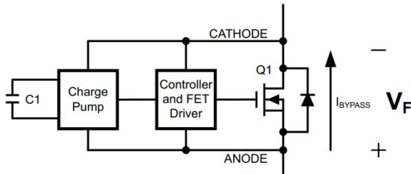
“Smart Diode” TO-263-3 and function diagram.
