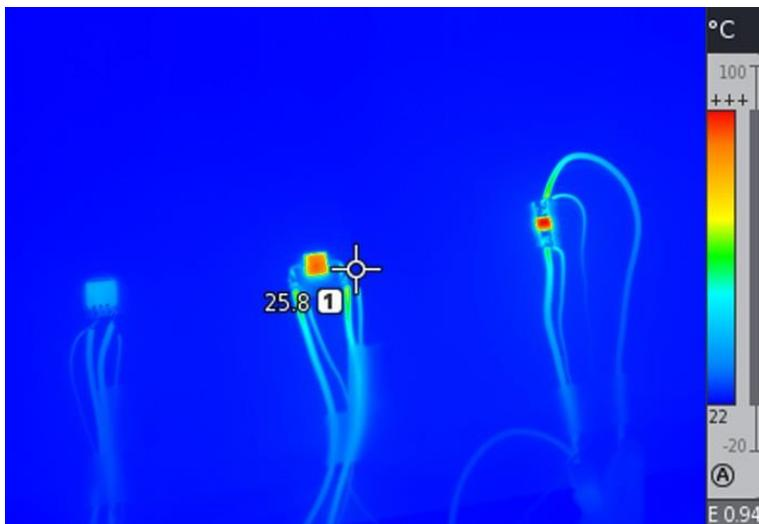
Figure 5 Thermal image seen from the back. Highest surface temperature is more than 100 degC. Current = 5A.
