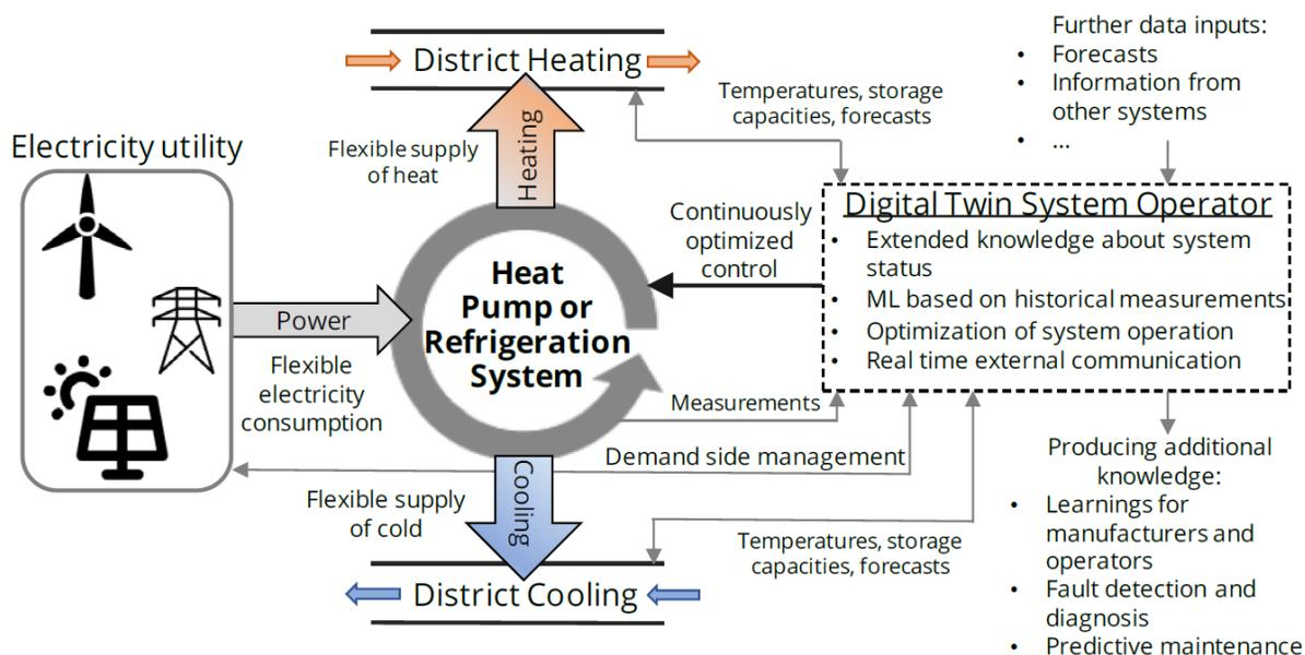
Figure 1: Diagram of the digital twin system operator.
