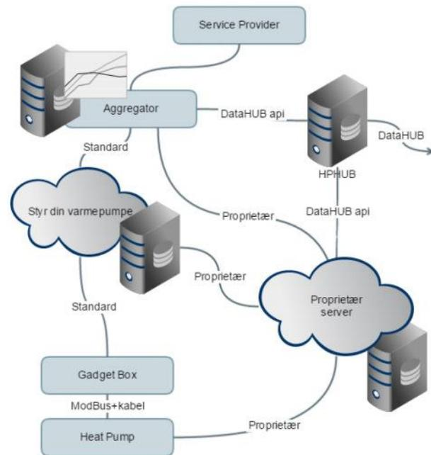
Figure 2: Principle for heat pump datahub (high level).
