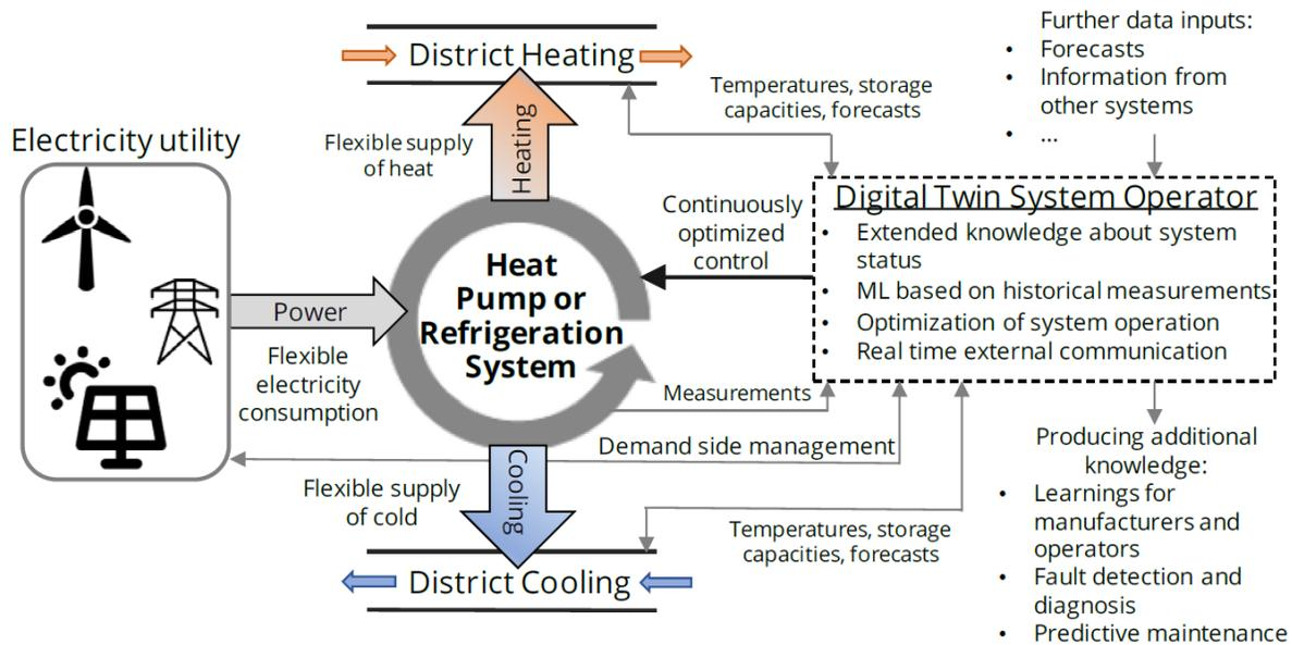
Figure 12. Diagram of the digital twin system operator.
