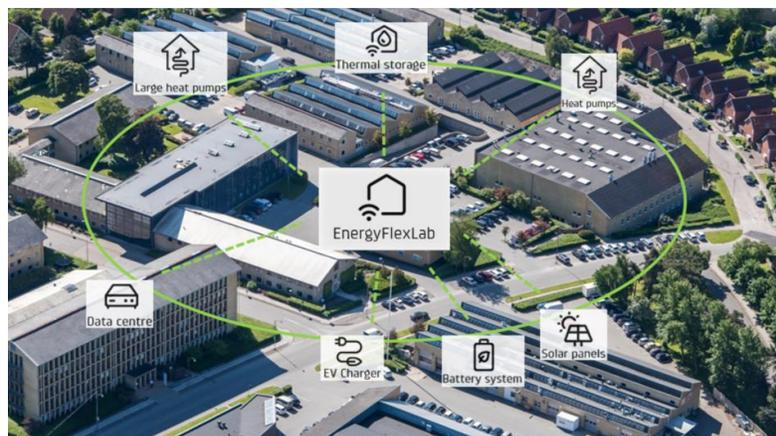
Figure 10. Main energy components in EnergyFlexLab.
