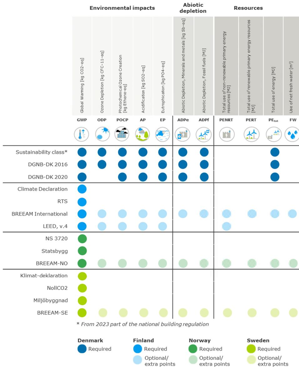
Figure 3 - Different impact categories included in the LCA calculation (required and optional) for the different certification schemes and legislation across the Nordic countries; Denmark, Finland, Norway and Sweden. For BREEAM International, BREEAM-SE and BREEAM-NO only GWP is required to document. Because it is optional which two additional impact categories are addressed it is possible that impact categories besides the above listed would be addressed.
