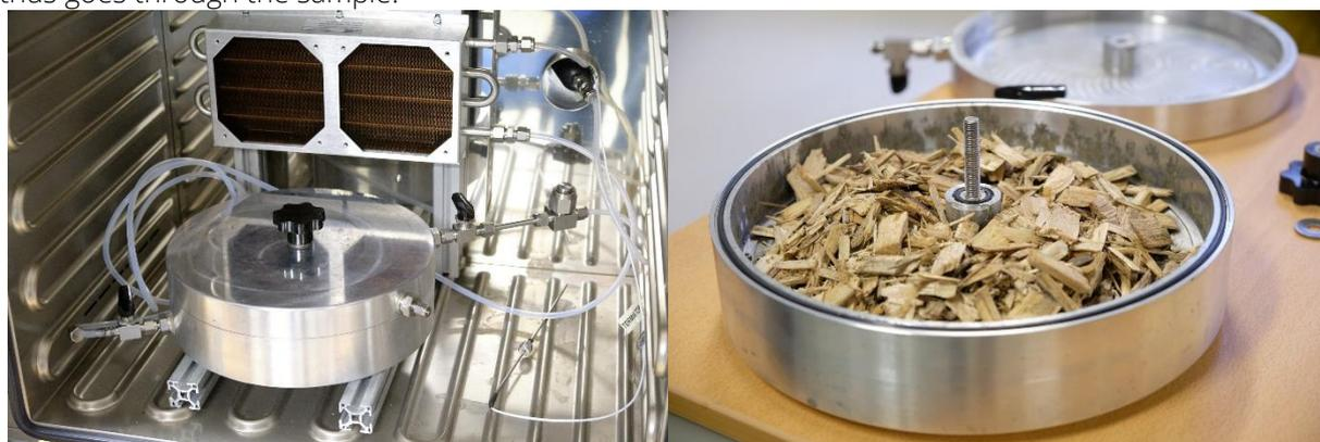
**Figure 2** Left: Sample chamber installed in the oven of the primary standard. The gas inlet is installed in the bottom of the chamber on the left, and the outlet is installed in the top of the chamber on the right. Right: View of the open sample chamber with wood chips placed on top of the built-in sieve.
