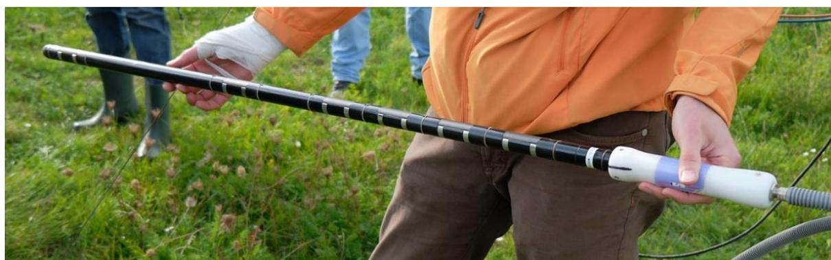
**Figure 4** Soil moisture sensor that produces moisture readings at different depths at the same time.
